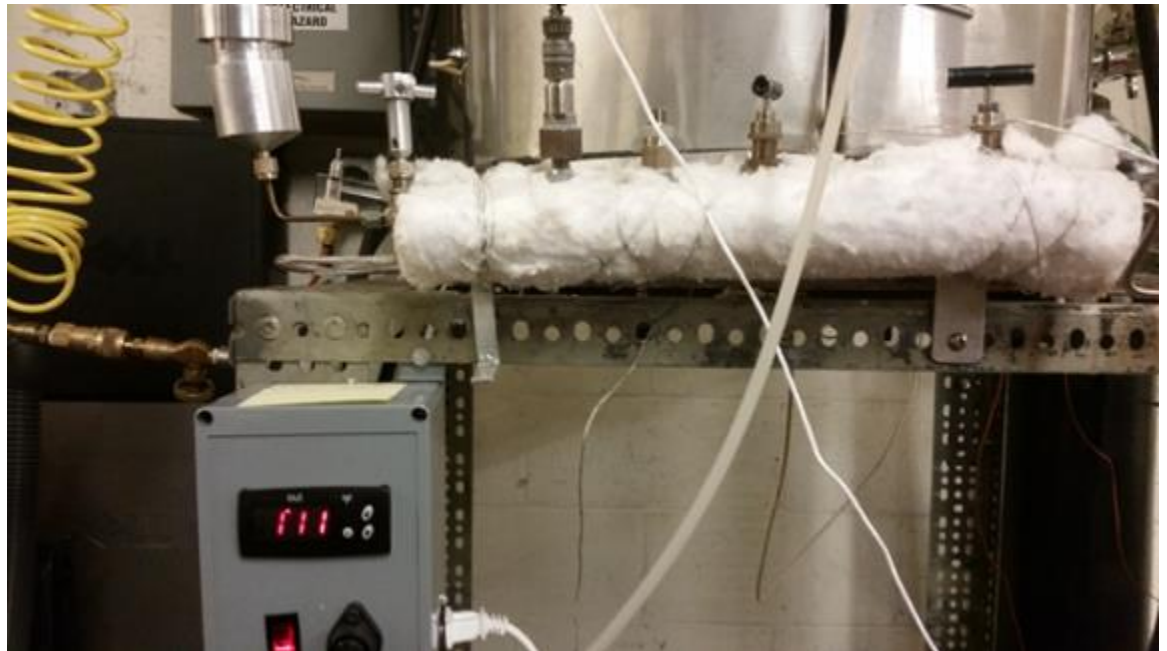
Figure 17: Heated liquid filling lines and controller
