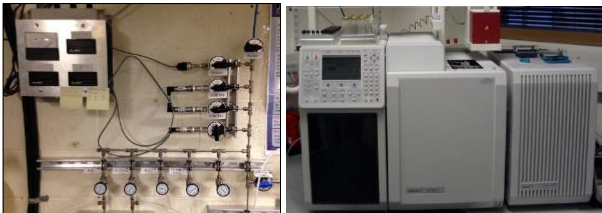
Figure 5: Image of partial pressure filling system and Gas Chromatograph
